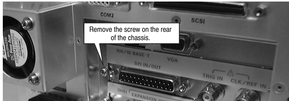
Figure 5: Removing the screw on the rear of the chassis
